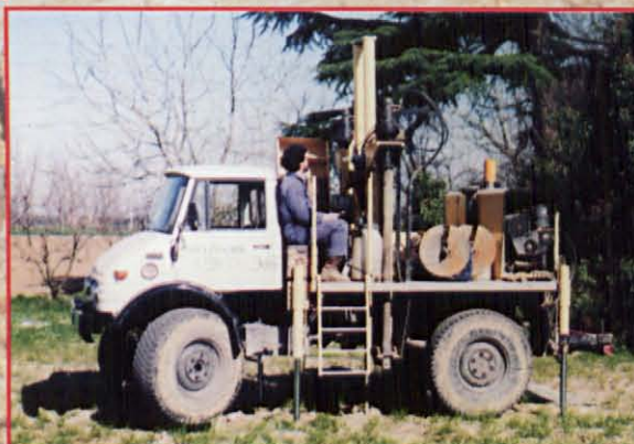
PENETROMETER TG 73-200 kN STATIC-DYNAMIC- ROTARY
