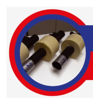
New high conductivity borehole filling (grouting) materials, including low temperature PCM\*
