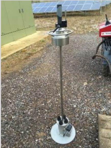
Figure 1. Components of the Light Falling Weight Device (LFWD)
